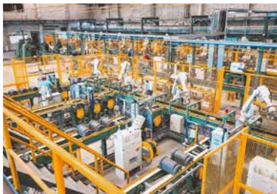
➤ Robots for production roof cover
