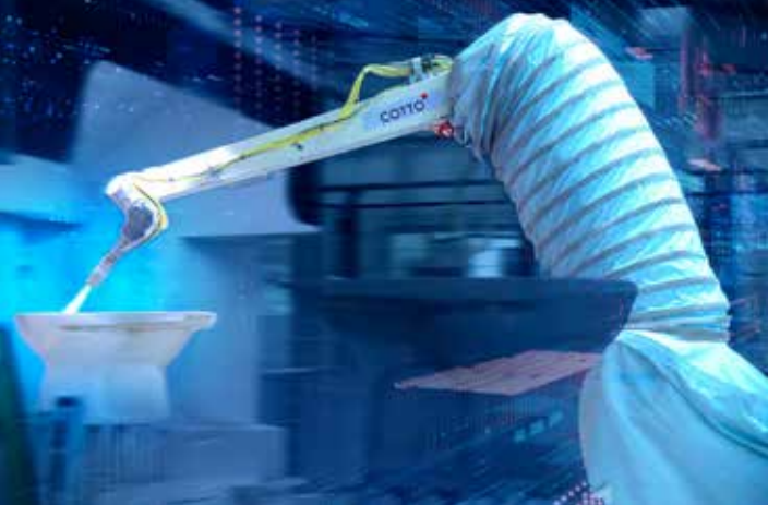
➤ An automated robotic spray painting system to enhance production efficiency swiftly
